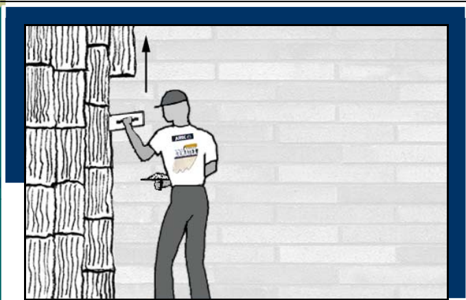
(diagram.2) transfer texture to the wall
