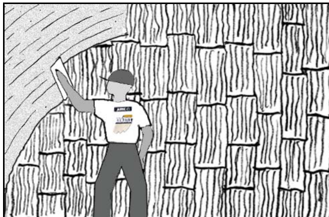
(diagram.3) smooth off and remove excess
